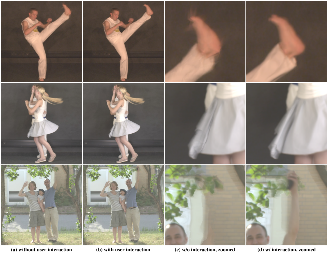
Figure 9: Morphed images from 8 views (4 cameras, 2 time steps). Row 1: Capoeira scene. Different artifacts in the views produce a halo streaking effect around the foot (c), while the corrected version features only minor motion blur (d). Row 2: Dancers scene. The blended skirt artifact (c) has vanished in the repaired version (d). Row 3: Family scene. Widely differing failure modes make the blended arm almost invisible (c), while the correct version preserves the arm’s shape.
